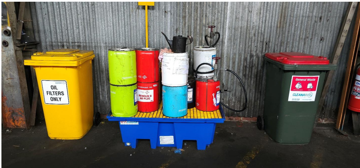
Plate 2 Waste receptacles, including inappropriate storage of drums
